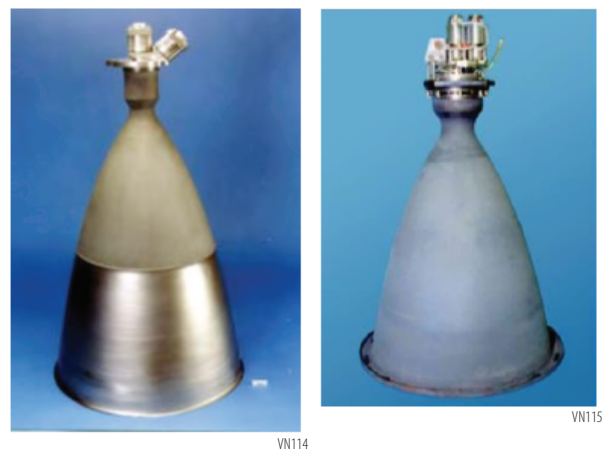
Figure B-108. R-40B 4,000N (left) and R-4D-15 450N (HiPAT, right) rocket engines (not to scale)
